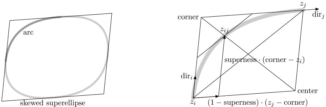
In order to draw such an arc, the user defines the starting points  $z_i$ , the starting direction  $\text{dir}_i$ , the ending point  $z_j$ , the ending direction  $\text{dir}_j$  and a so-called *superness*. The macro `arc(zi, diri, zj, dirj)` then defines the path as follows:
